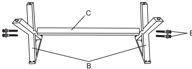
Setp 1: Install the fixed pole(C) onto 2pcs feet(B) by screws(E)and washer(G).
